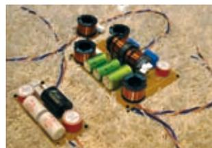
The three-part crossover (displayed here on the thick carpet of the listening room) is equipped with components from the respected supplier, Mundorf.
