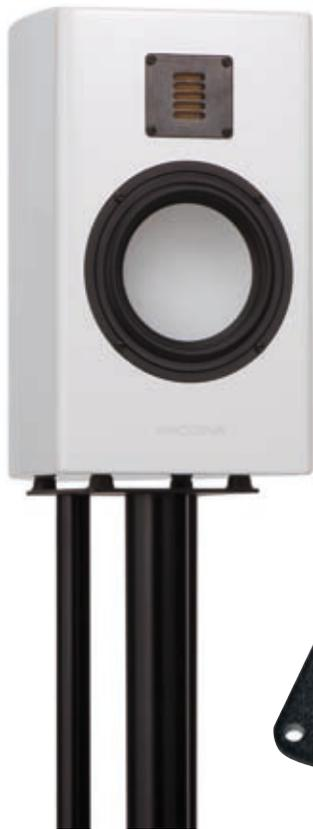
The recommended Gaudeer speaker stand (300 Euros / pair) is sand filled and 70 centimeters in height, which brings the Arcona 40 to exactly the right listening height. The AMT high frequency driver has enormous power reserves, 94 dB sensitivity, and shines because of its wide dispersion and small radiating surface.
